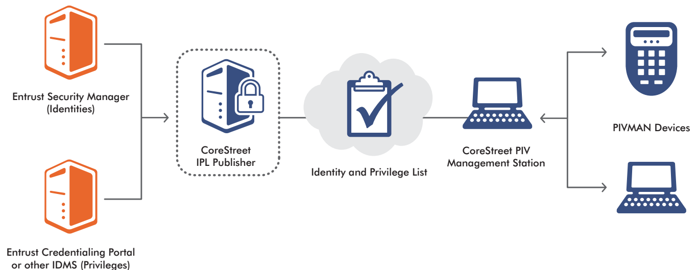
Figure 1: Described at a high level, the system registers users and issues identities (digital certificates). The identity information is mapped to privilege and characteristic data, including roles (as defined by DHS), and more granular information such as specialized training an individual may possess. This data is consolidated and transmitted to management stations and field authentication devices. Changes, updates and credential revocation are synchronized automatically and in real time, so the field devices always have the most recent data.
